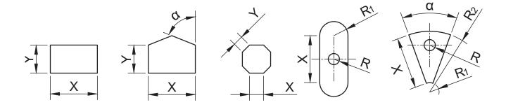
X - length, mm; Y - width, mm;  $\alpha$  - angle, °; R, R<sub>1</sub> and R<sub>2</sub> - radius, mm.
